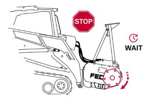
CONTACT WITH MOVING ROTOR CAN CAUSE SERIOUS INJURY OR DEATH. DO NOT EXIT THE VEHICLE BEFORE THE ROTOR STOPS.
